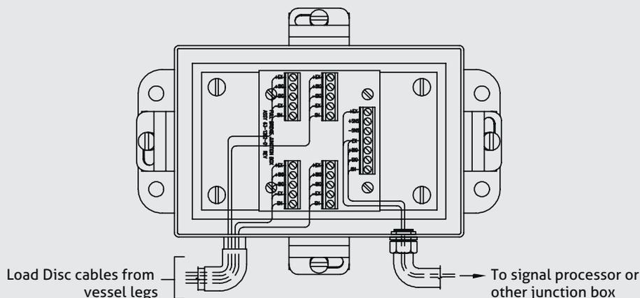
2. Pass the Load Disc cable through the desired connection. (See Figure 3-8).
